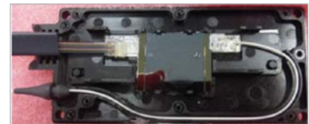
Figure 7: Layout of an AWG multiplexer and picture of an AWG chip inside a device
